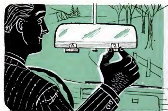
REAR-VIEW MIRRORS that can be easily re-aimed after they've been moved. Marked dials would let each driver of the car adjust the mirror to his own setting.— J. Nathan, Winnetka, Ill.
